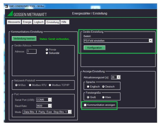
With the help of the tool the protocol can now be configured as desired. The protocol can be adjusted by ticking the desired parameters. The following figure shows the setting for the standard telegram. The settings can be saved in the PC with "Store".
